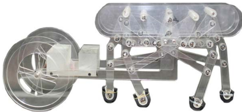
Figure 1.7 Chiang's 10-link type wooden horse carriage [14]
